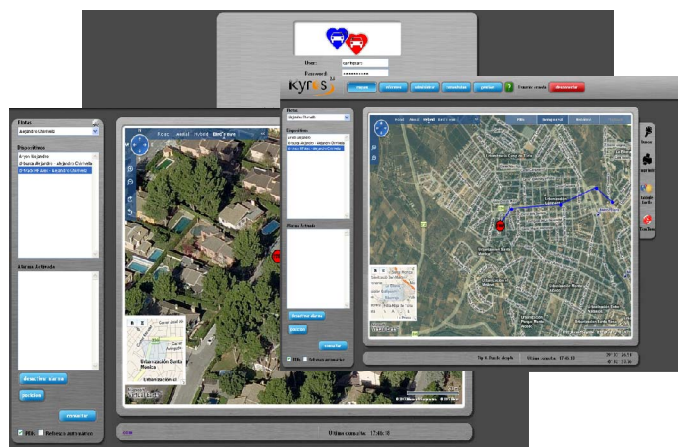
Figure 8. The PSAP web application shows the crashed car location and tracking
