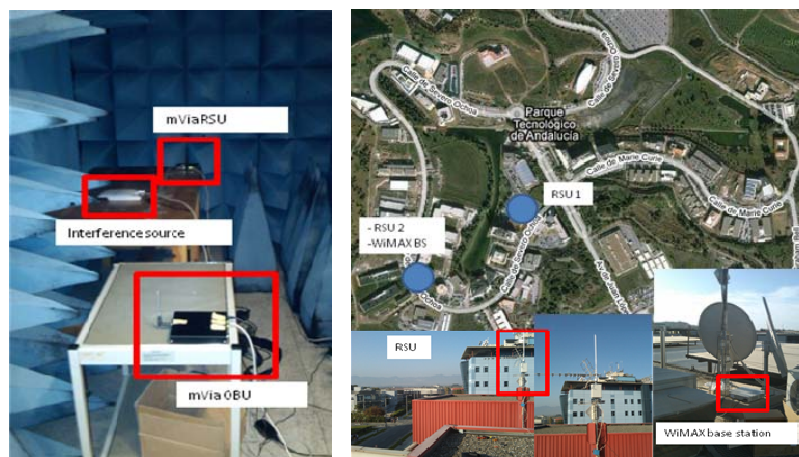
Figure 2: Bench test set-up (left) and field testing area with RSU deployment (right)
