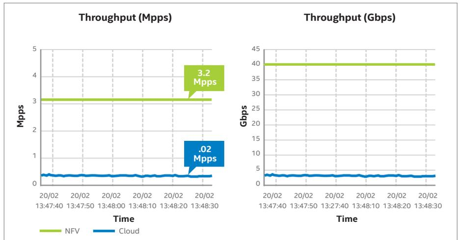
Figure 6. Performance Comparison for 1518 byte frame size.
