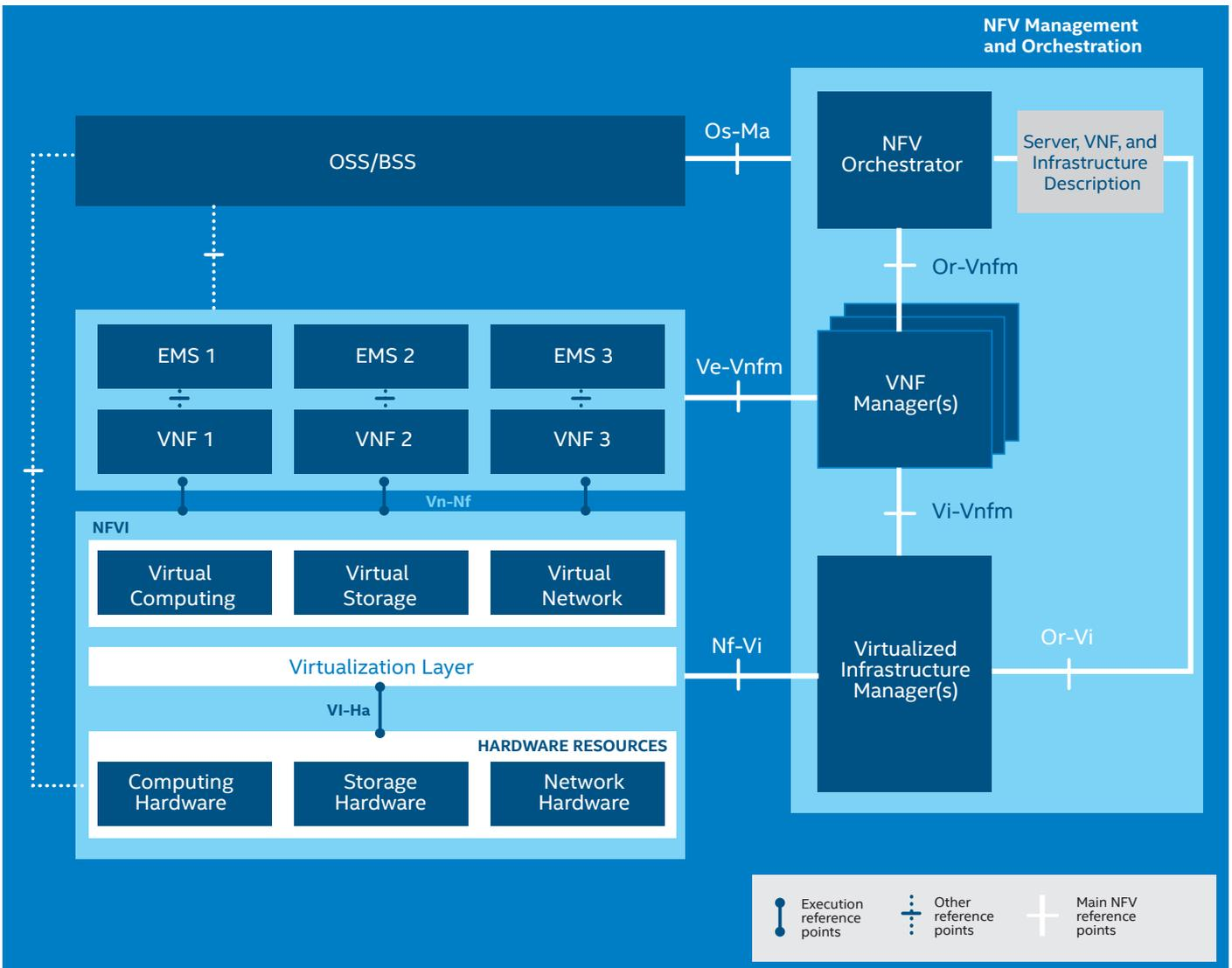
Figure 1. ETSI End to End NFV Architecture.
